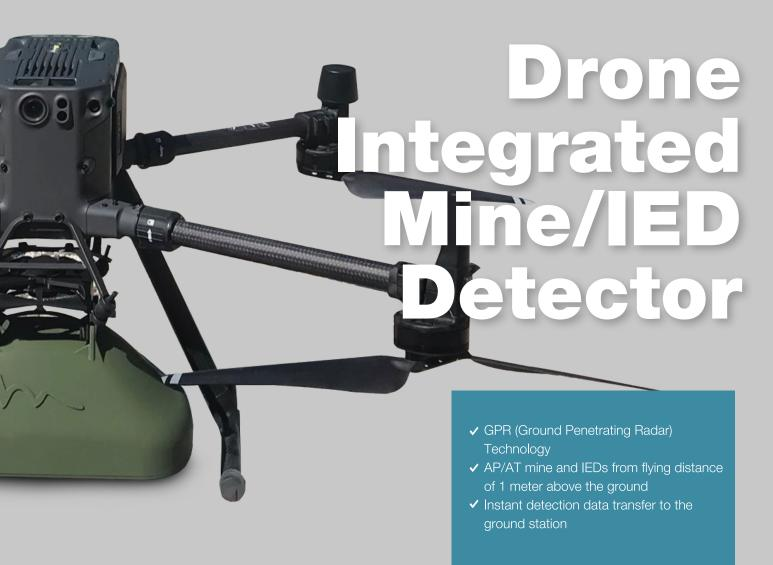
MeDro allows Counter-IED teams to operate with full safety having the advantage of GPR tech, being integrated to a drone. With its advanced innovative detection technology, it enables the aerial detection of IEDs and mines.
